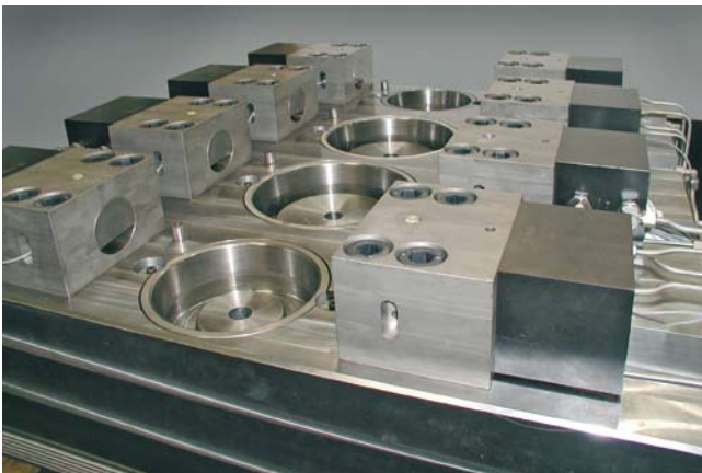
Wedge clamp in a forging die Temperatures up to 250°C
