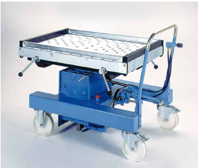
Die cart, manually operated, type DL with foot pump or electro-hydraulic lifting
